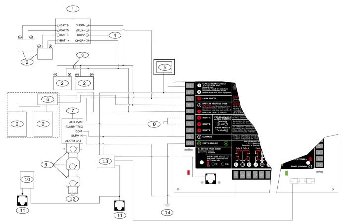
Figure 3.2: Side System Wiring Diagram
